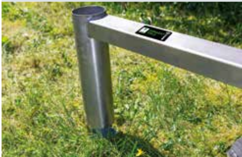
Post setting gauge for precise post spacing with height adjustment for sloping or uneven terrain
